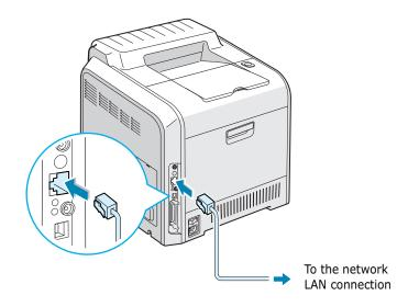
**10** Connect the network cable, reconnect the power cord and then turn the printer on.
